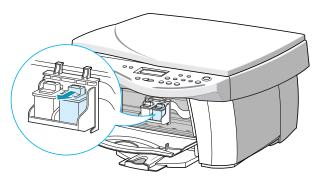
5 Place the new print cartridges into the holder and push it until it clicks into place.
